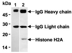
Immunoprecipitation of Histone H2A from HeLa cells with mouse IgG2b (1) or D210-3 (2). After immunoprecipitated with the antibody, immunocomplex was resolved on SDS-PAGE and immunoblotted with D210-3.
