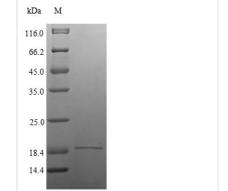
(Tris-Glycine gel) Discontinuous SDS-PAGE (reduced) with 5% enrichment gel and 15% separation gel.
