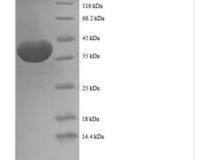
(Tris-Glycine gel) Discontinuous SDS-PAGE (reduced) with 5% enrichment gel and 15% separation gel.
