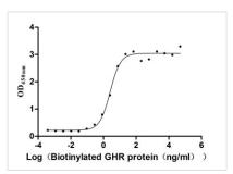
Activity Measured by its binding ability in a functional ELISA. Immobilized human GH1 at 2 μg/ml can bind Biotinylated human GHR (CSB-MP009411HUj1-B), the EC<sub>50</sub> is 2.067-3.208ng/ml.
