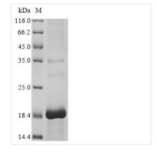
(Tris-Glycine gel) Discontinuous SDS-PAGE (reduced) with 5% enrichment gel and 15% separation gel.
