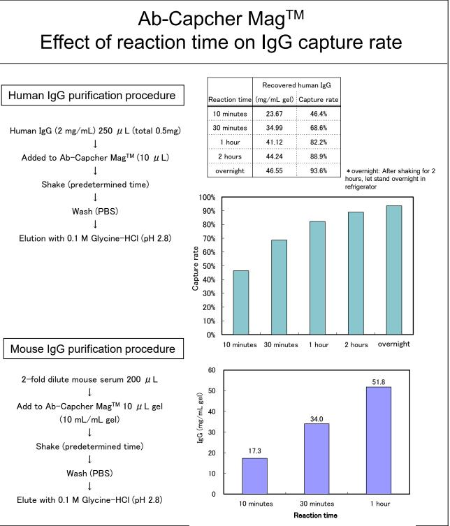
Ab-Capcher Mag<sup>™</sup> was studied to determine the effect of reaction time on the amount of purified antibody and its rate of capture. For human IgG, yield increased with increasing reaction time: 82% in 1 hour and 89% in 2 hours. By allowing the reaction to stand overnight (4° C), it was possible to recover 90% or more of IgG. For mouse IgG the amount of purified antibody also increased with increasing reaction time, with 51.8 mg/mL gel IgG purified in 1 hour.
