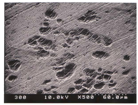
Fig. 3 Pit on the slice of ivory. (SEM picture)
