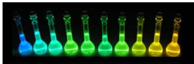
Fig1. Emission spectra change of solvatochromic fluorophore
