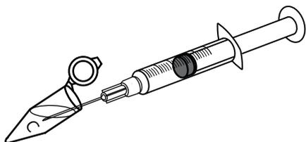
5. Remove the needle from the syringe and connect the filter unit to the syringe.
