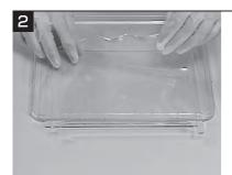
Hold both lower corners of the gel and gently peel it away from the glass plate.
