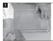
Hold the gel plate with the shorter glass plate facing upward. Insert a spatula or similar tool between the plates and twist gently to remove the glass plate. Make small cuts at both ends of the gel along the spacers.
