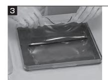
Carefully lift the gel and immerse it in the CBB staining solution.
