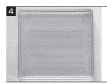
Stain for approximately 1 hour with gentle shaking, then replace the solution with destaining solution.
