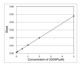
Figure 3: Calibration curve by kinetic method (30 minutes incubation)
