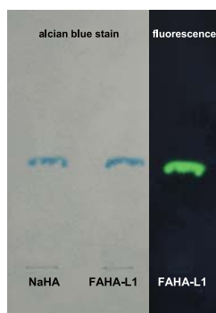
Cellulose acetate membrane electrophoresis of FAHA-L1
