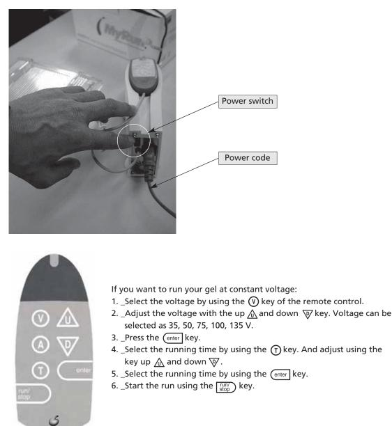
If you want to run at a constant ampere, apply the same procedures using the A key instead of V (20, 30, 40, 50, 60, 70, or 80 mA can be selected).
