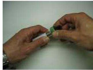
2. By turning the upside small knob to the right, the internal O ring will be extended, and the tube will be sealed completely.
