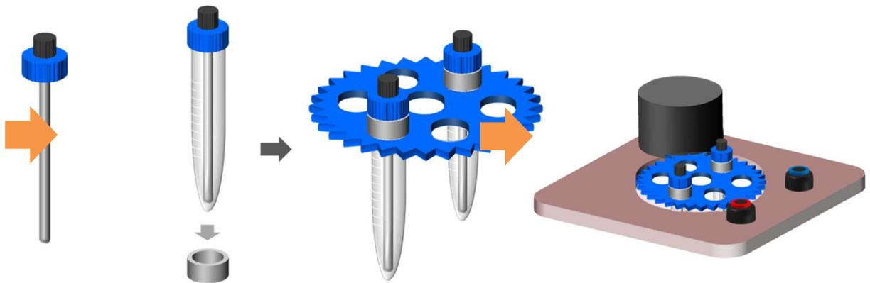
1. A resonance rod unit is inserted in the tube of the sample and the screw cap is turned to the right, closing.
