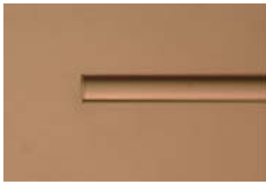
[The end of a glass capillary pipette prior to polishing]
